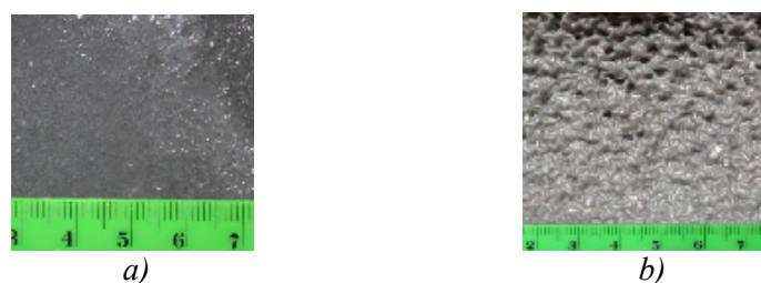
Fig. 12. The effect of film thickness on the quality of the inner surface ( \text{HEMA}:\text{PVP}:\text{H}_2\text{O}=70:30:100X_w , [\text{Zn}]=20\text{ wt}\% ; \omega=700\text{rev}/\text{min} ): a – 1 mm, b – 4mm
